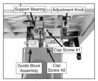
Figure 30. Side of lower blade guide.
